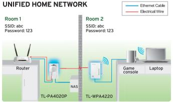
\*The powerline adapters need to be connected in the same electrical circuit.
