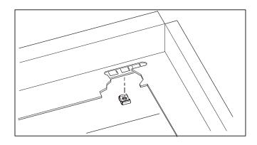
3. Fasten the duct and bellow assembly to the rail assemblies using two, M6 ×12 mm, Phillips pan-head screws and the caged nuts installed in last step.
