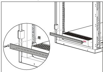
**Other openings** For proper operation and maximum cooling, all other openings in the enclosure should be covered using standard blanking plates—(not provided).
