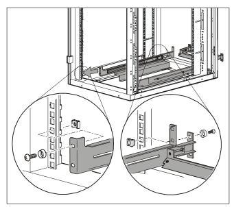
8. After the rails are in position retighten any nuts loosened in step 4.
