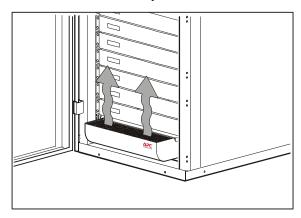
When to use<br/>only one fanDepending on your enclosure's height and the heat output of<br/>installed equipment, you may choose to operate only one fan,<br/>thus reducing energy consumption. Smaller enclosures often<br/>require only one operating fan.You may also choose to operate both fans during normal<br/>operation, and turn off one fan in the event of a loss of utility<br/>power. This will conserve run-time on the battery of the UPS.
